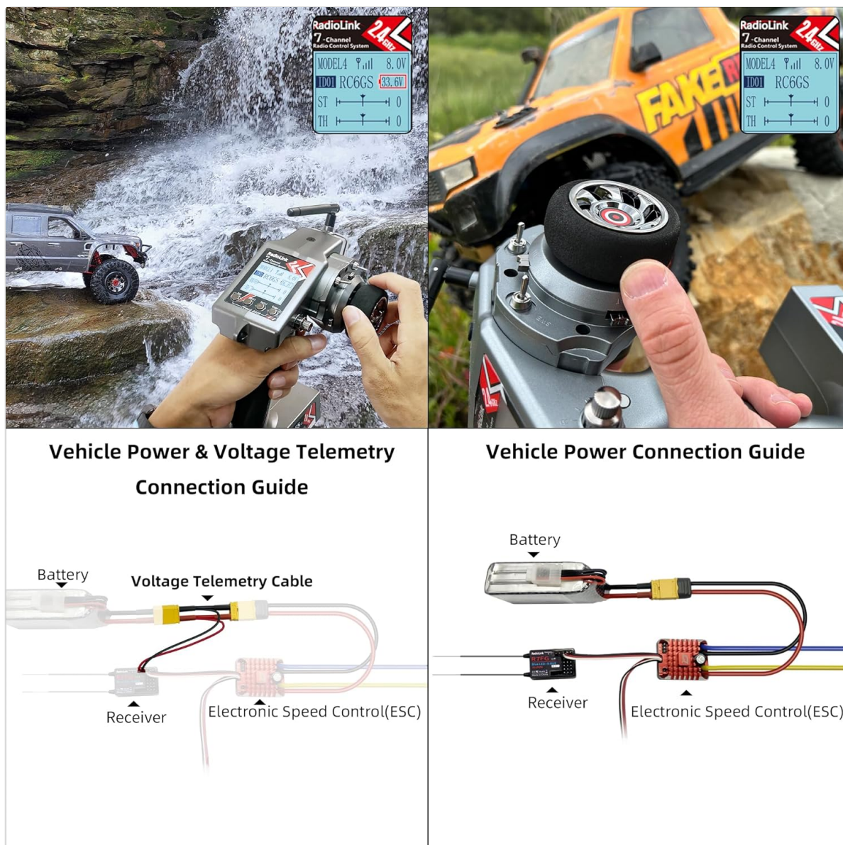
Figure 4: Vehicle Power and Voltage Telemetry Connection
