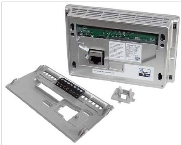
Image: The rear of the Trane ComfortLink II XL850 thermostat, displaying the terminal block for wiring connections and internal circuitry. The mounting plate is shown detached.
