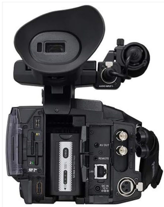
Figure 2.1: Rear view of the camcorder, highlighting battery and SD card slots.
