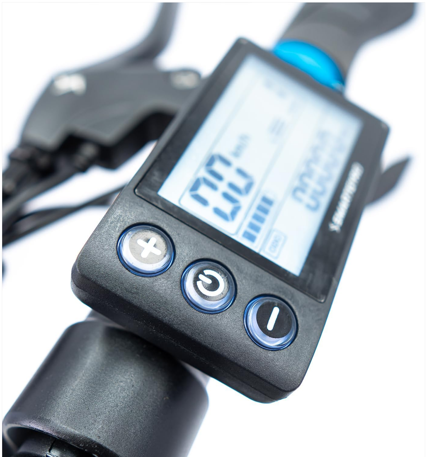
Image: A close-up of the handlebar display, showing speed, battery indicator, and control buttons for power and mode selection.
