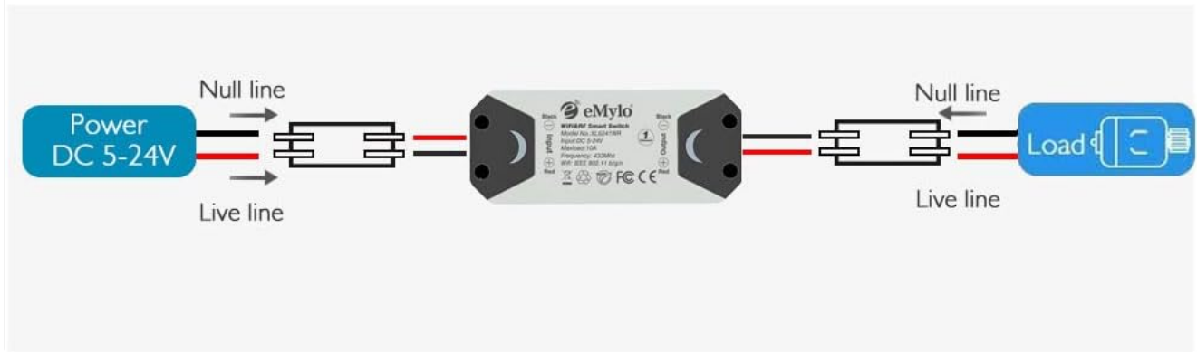
Image: Wiring diagram illustrating the connection of a DC 5-24V power source and a motor load to the eMylo controller module using push-in terminals.
