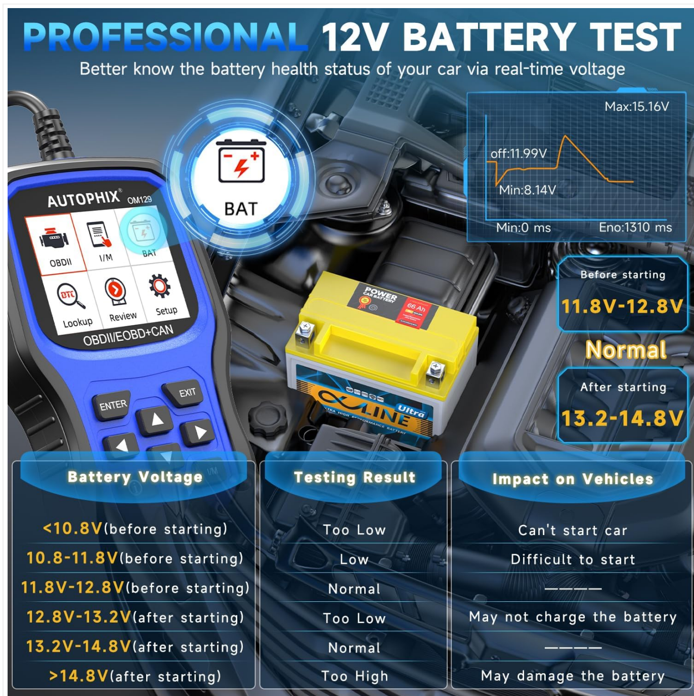
Figure 5: The OM129's battery test interface, showing real-time voltage graphing and a table indicating battery health based on voltage readings before and after starting the engine.
