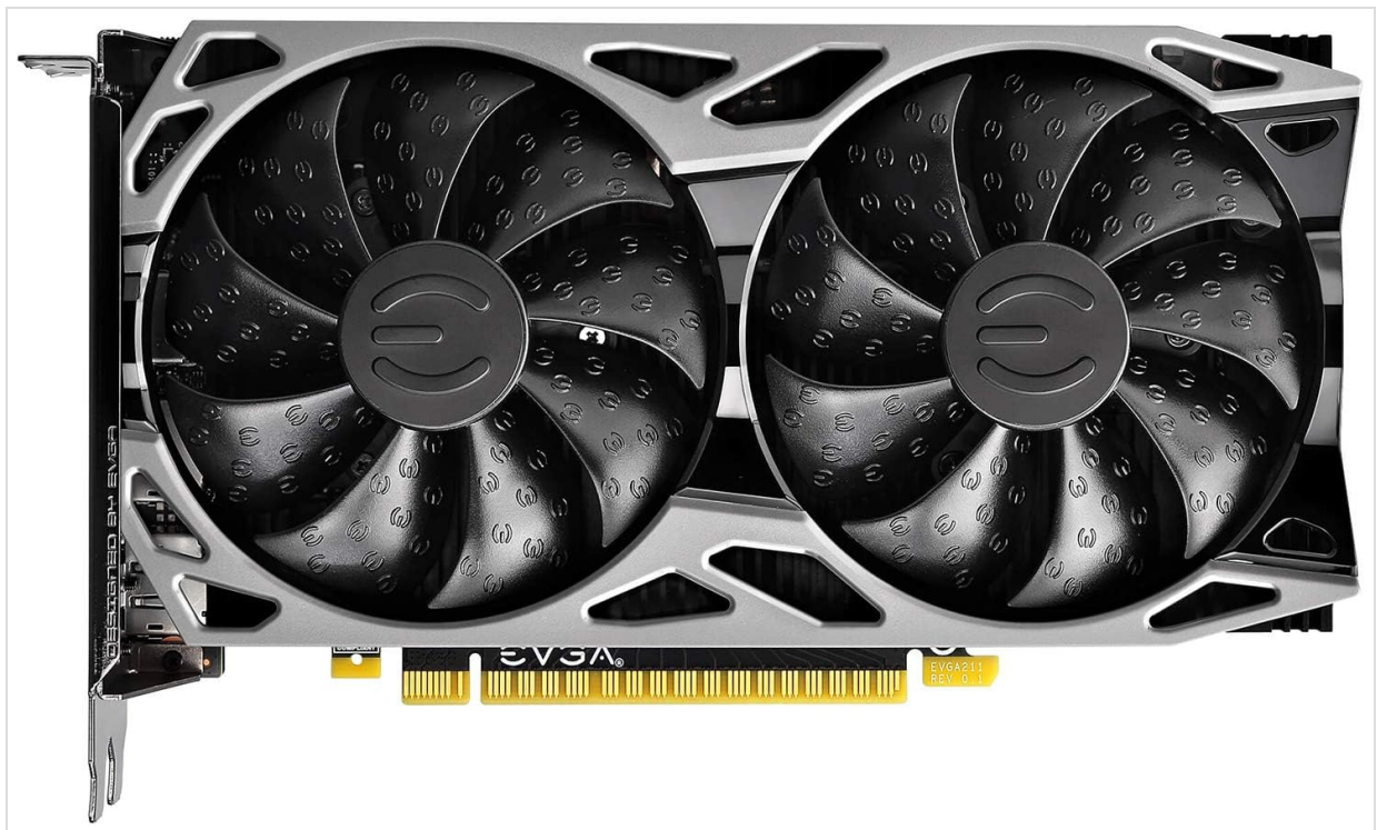
Figure 1: Front view of the EVGA GeForce GTX 1650 SC Ultra Gaming Graphics Card, highlighting the dual fan design.
