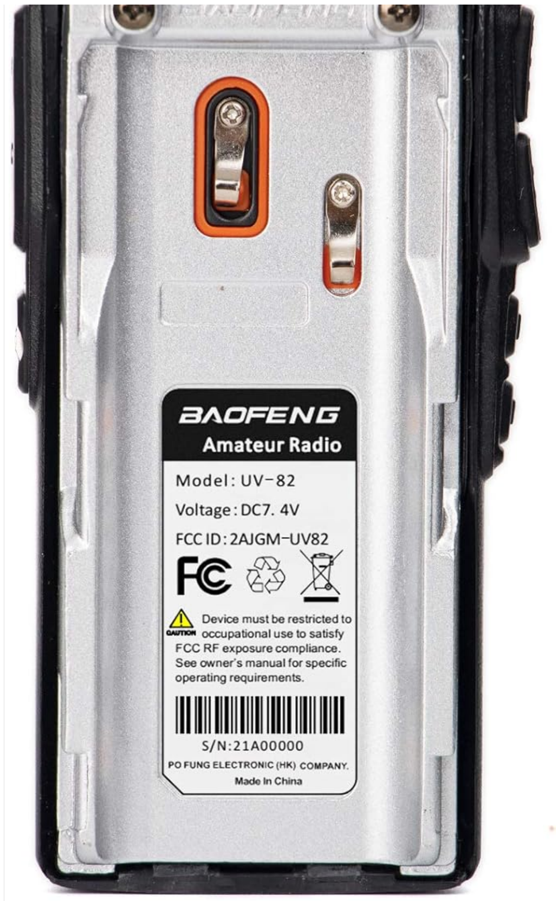
Image: Rear view of the BAOFENG UV-82 radio, detailing the battery contacts and regulatory information label, including the model number and FCC ID.
