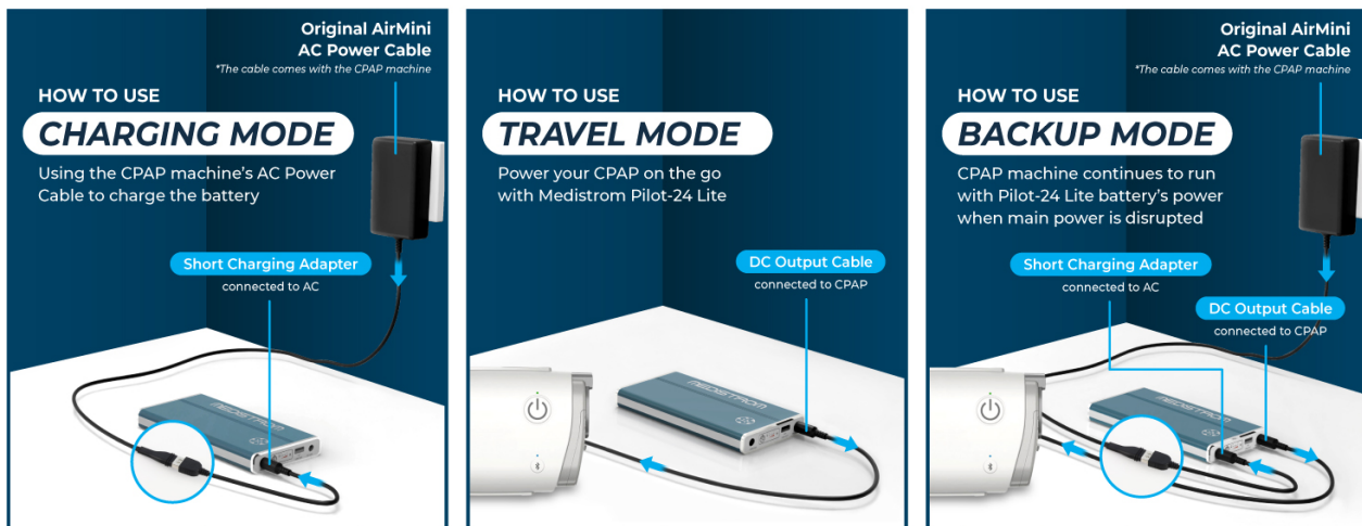
Figure 10: Illustration of the charging mode for the Pilot-24 Lite using the original S9 AC Power Cable.
