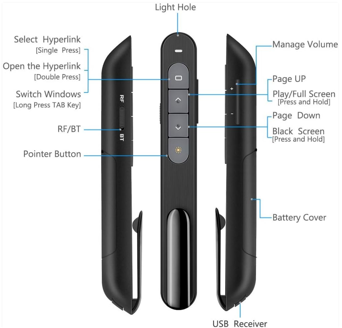
Image: A detailed diagram of the presenter, labeling each button and component, including the pointer button, page up/down, volume controls, and the RF/BT switch.
