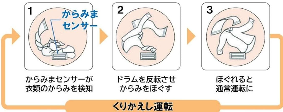
Image: Anti-Tangling Sensor. This visual guide demonstrates the anti-tangling sensor's operation, from detection to drum reversal and untangling.
