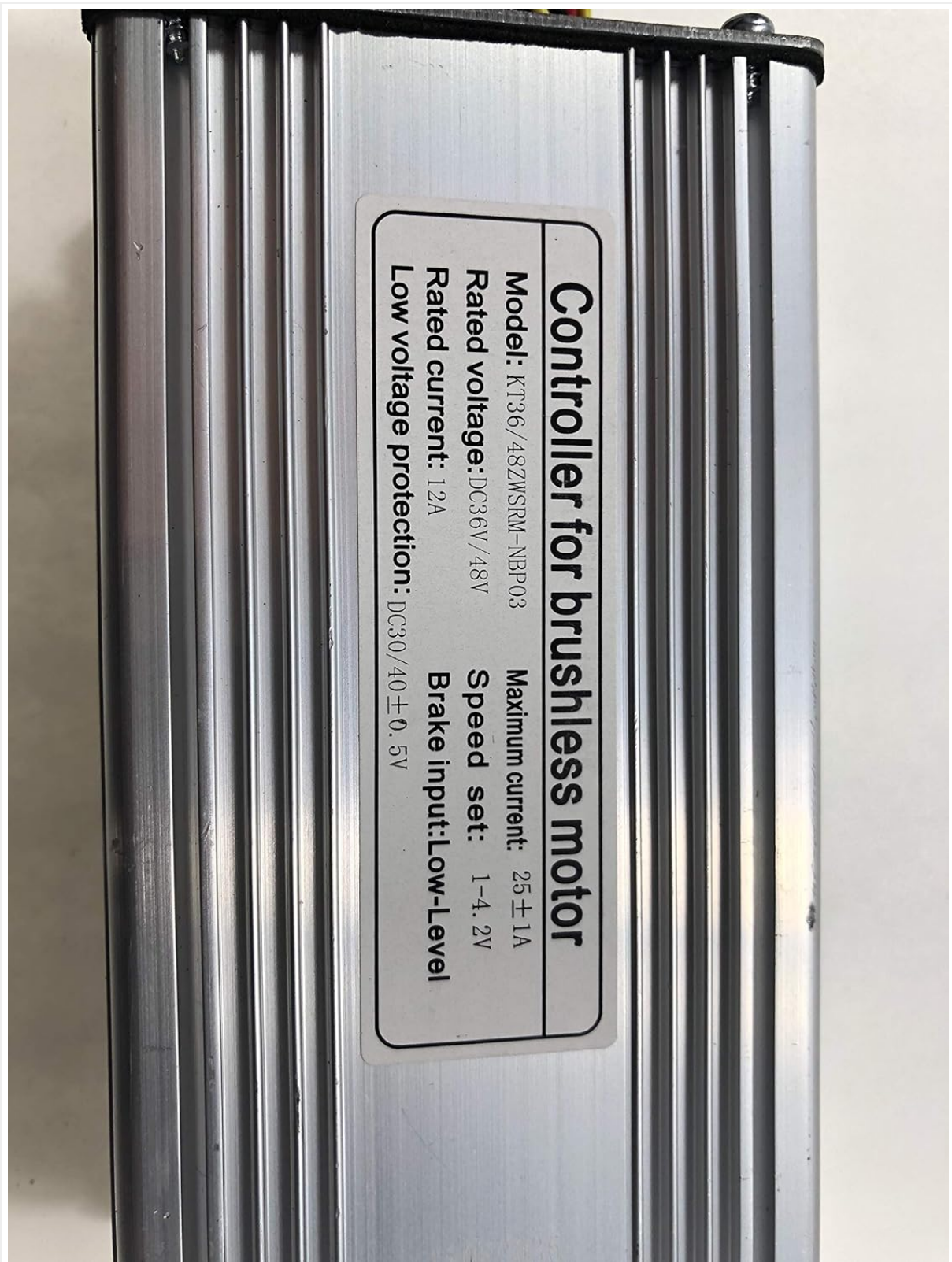
Figure 2: Controller label detailing technical specifications.
