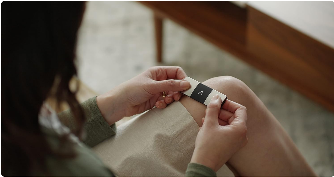
Figure 2.1: Proper placement of the KardiaMobile 6-Lead on the knee for a reading.
