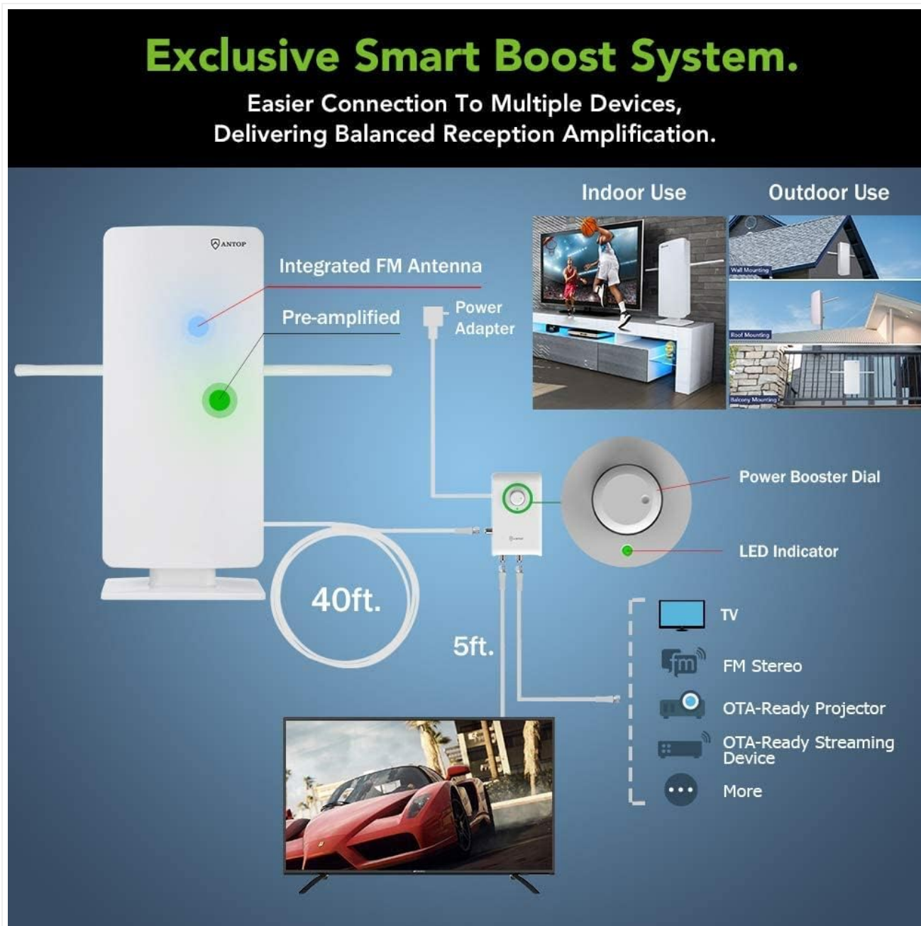
Image 4.1: A diagram illustrating the connection of the antenna to the Smart Boost System and then to a television or other devices.
