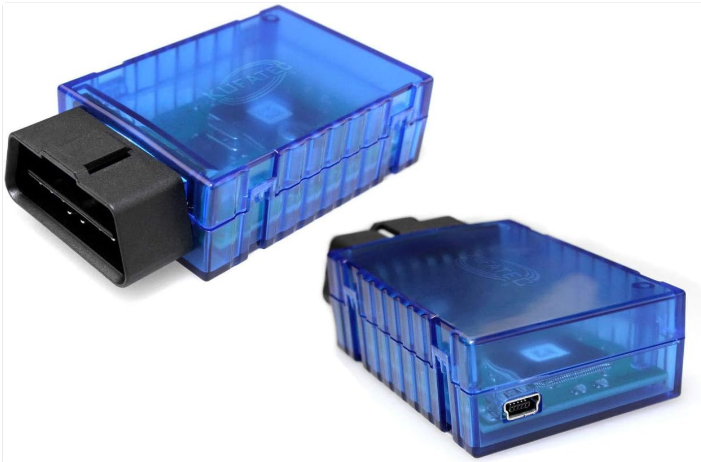
Figure 1: Kufatec LED Taillight Coding Dongle with its OBD-II connector, ready for vehicle connection.
