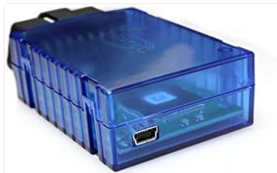
Figure 3: Side view of the Kufatec Coding Dongle, illustrating the mini-USB port which may be used for future software updates.
