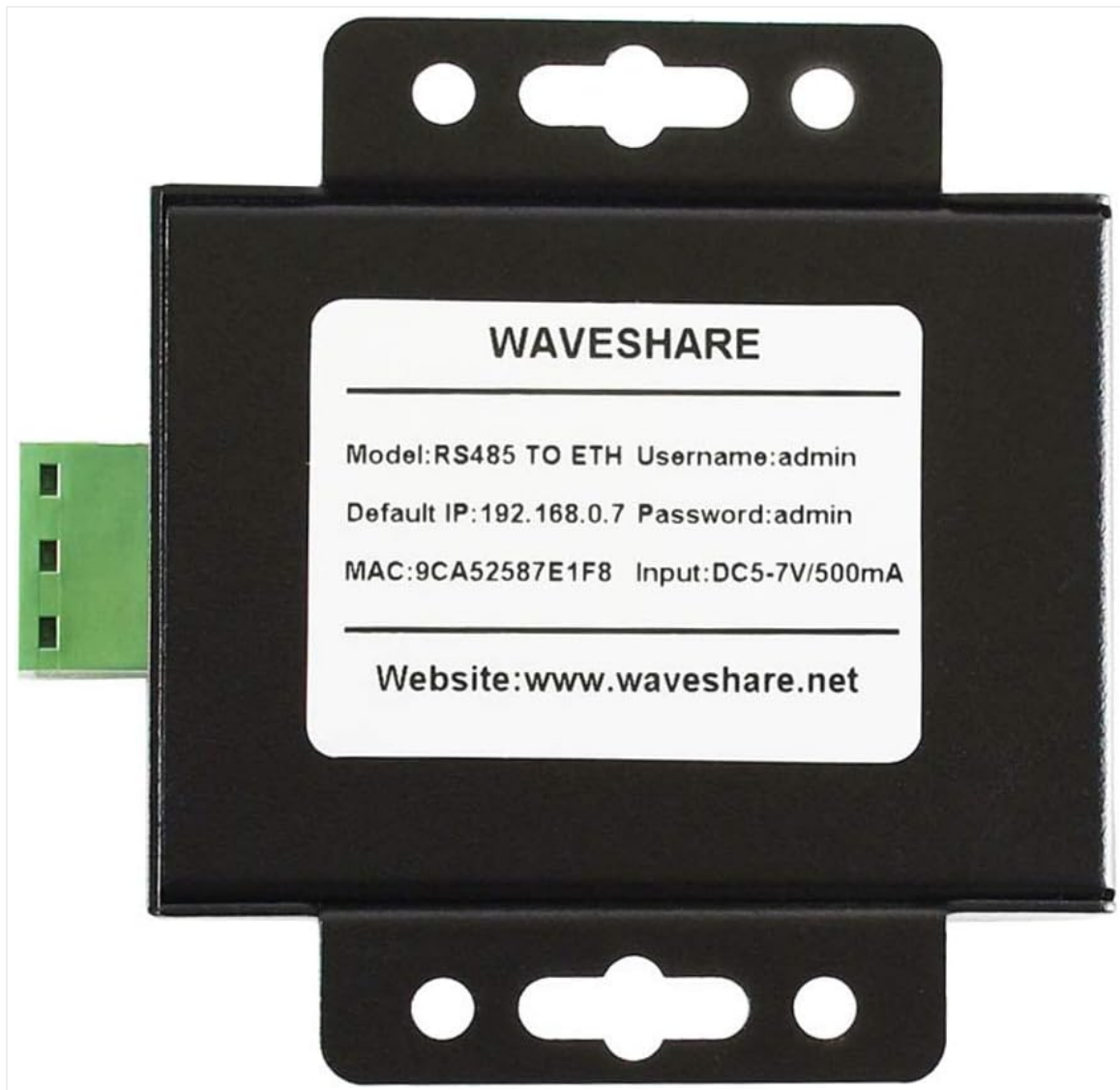
Figure 2: Bottom label of Waveshare RS485 to Ethernet Converter showing default network settings. The bottom of the converter unit displays a label with essential network configuration details: Model: RS485 TO ETH, Username: admin, Default IP: 192.168.0.7, Password: admin, MAC address, and Input power requirements (DC5-7V/500mA). The manufacturer's website, www.waveshare.net , is also listed.
