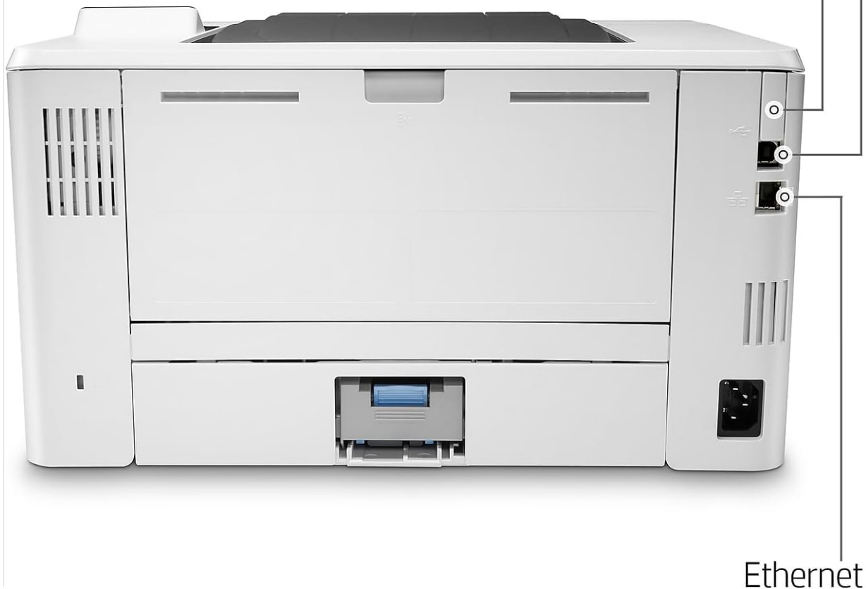
Rear view displaying USB 2.0 and Ethernet ports for connectivity.
