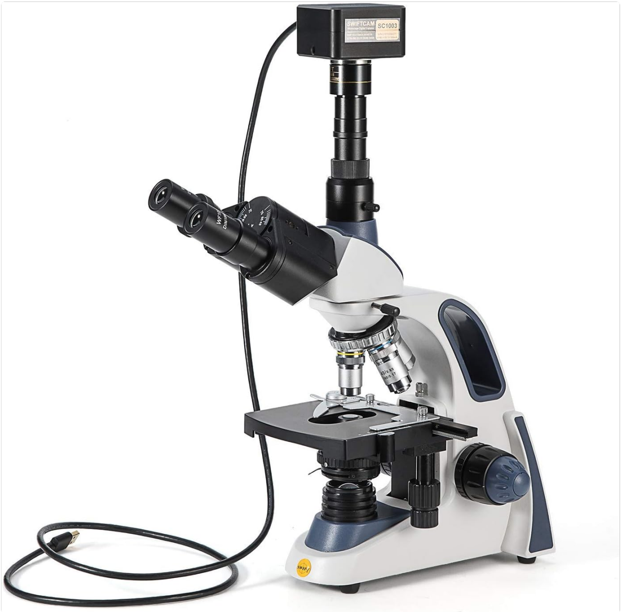
Image: The SC1003-CK camera properly mounted on a trinocular microscope, ready for use.
