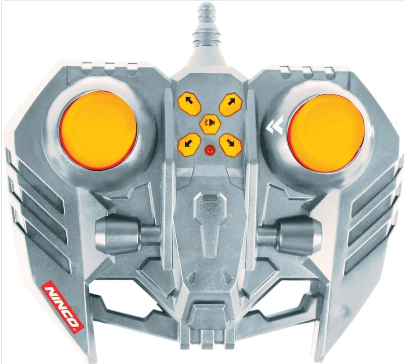
Figure 3.2: The 2.4 GHz remote control for the Ninco Driftrax RC Car, showing its dual joysticks and directional buttons.
