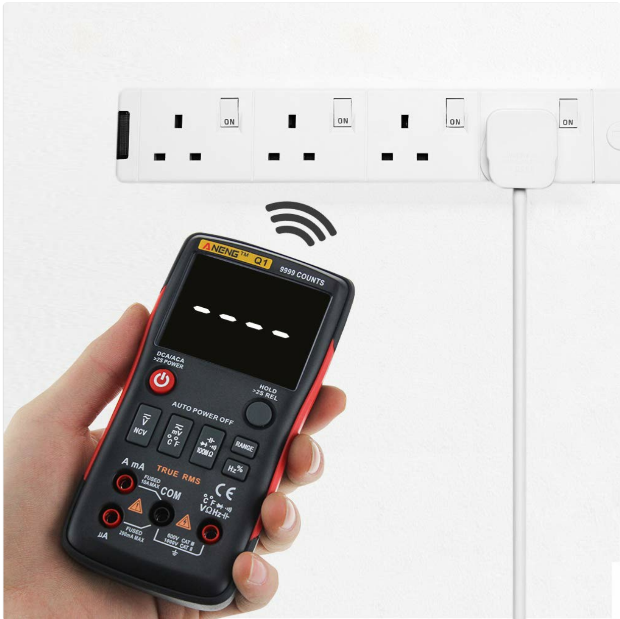
Image 5.1: The multimeter performing a Non-Contact Voltage (NCV) test near a power strip, indicated by the signal icon on the display.
