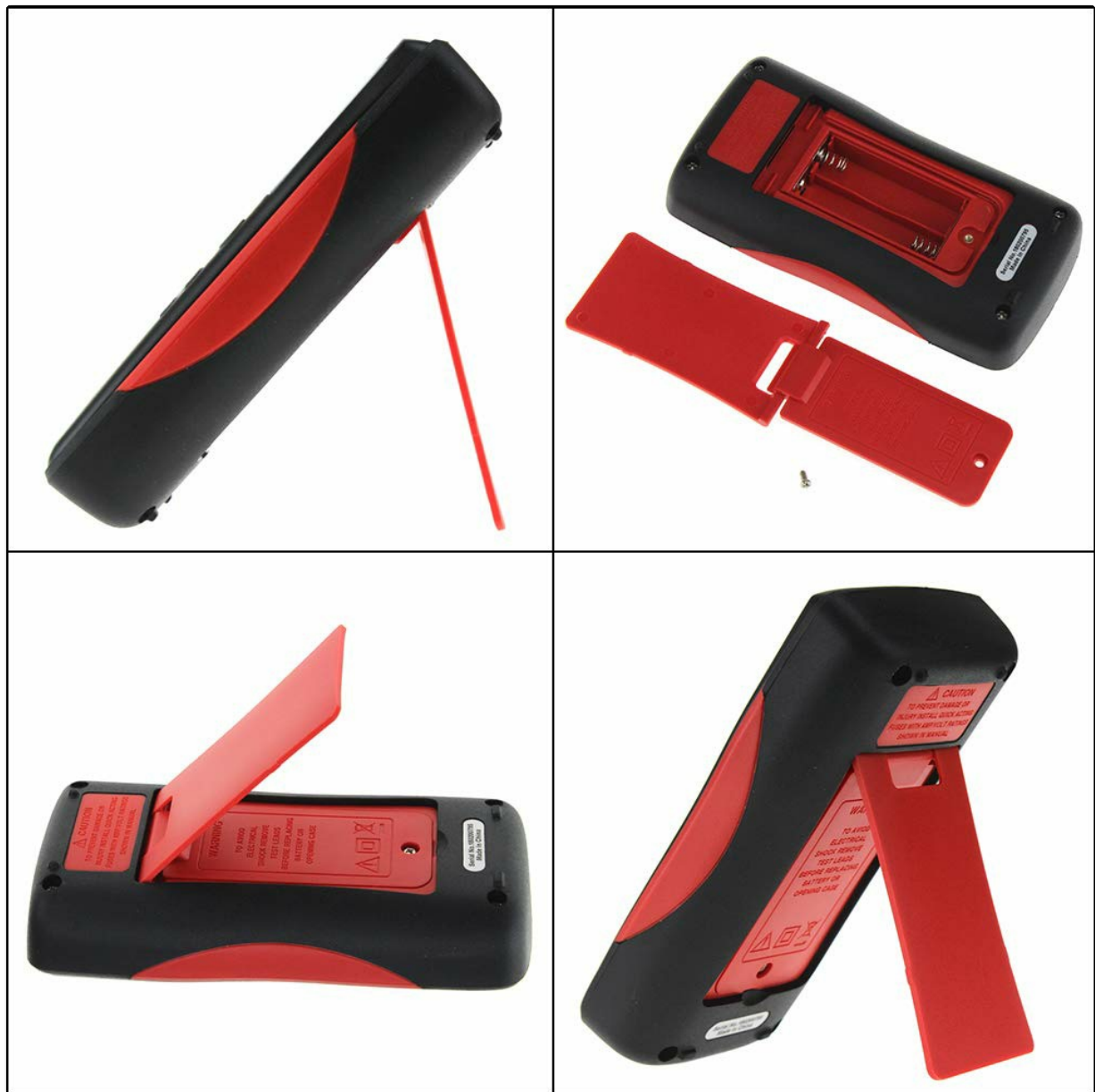
Image 4.1: Rear view of the multimeter, illustrating the battery compartment and the integrated kickstand.
