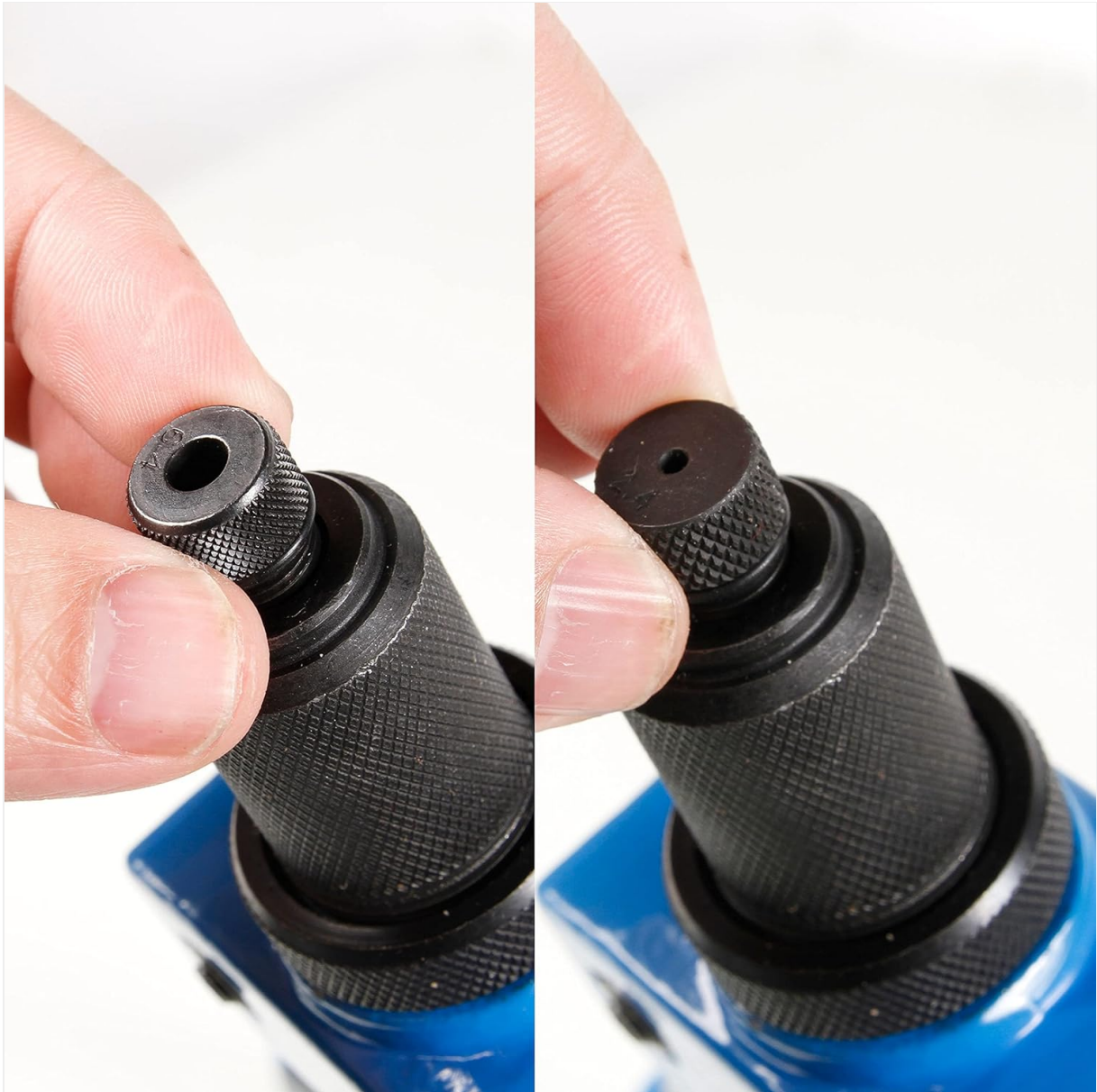
Image: A hand demonstrating the process of screwing an interchangeable nozzle onto the rivet gun head.
