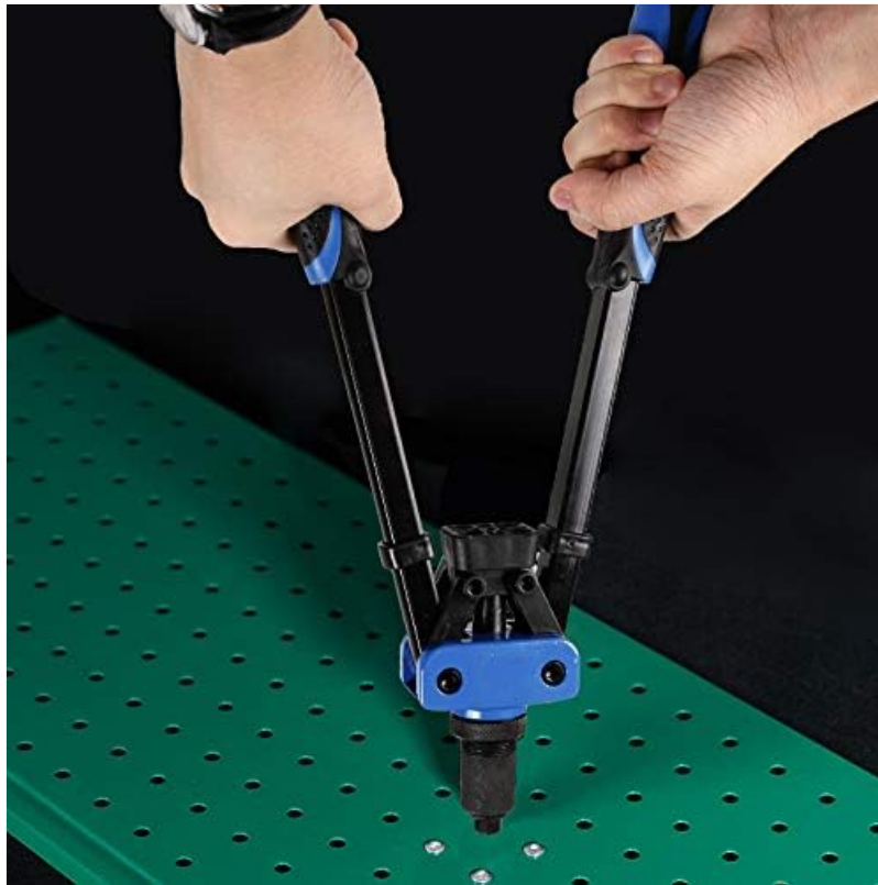
Image: A user operating the CCLIFE Rivet Gun to fasten a rivet into a green perforated panel.
