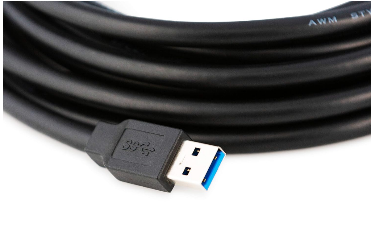
Image 2: A close-up view of the USB 3.0 male connector, highlighting its blue interior and the USB SuperSpeed logo.
