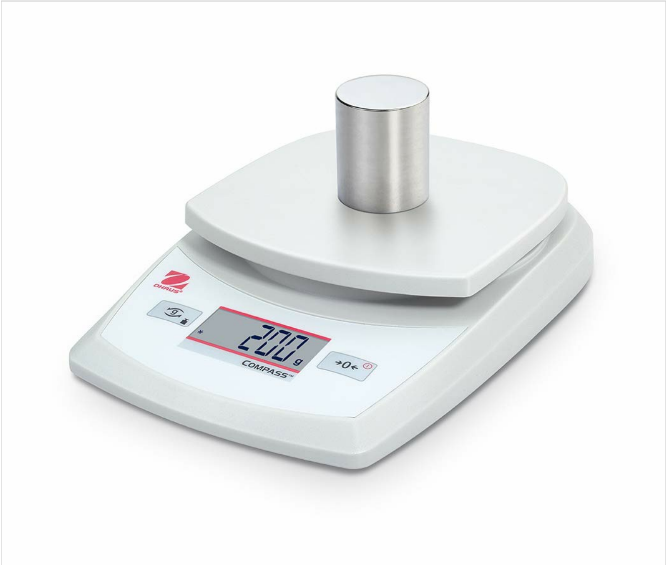
Image 4.2: The balance with a cylindrical calibration weight placed on the weighing pan.
