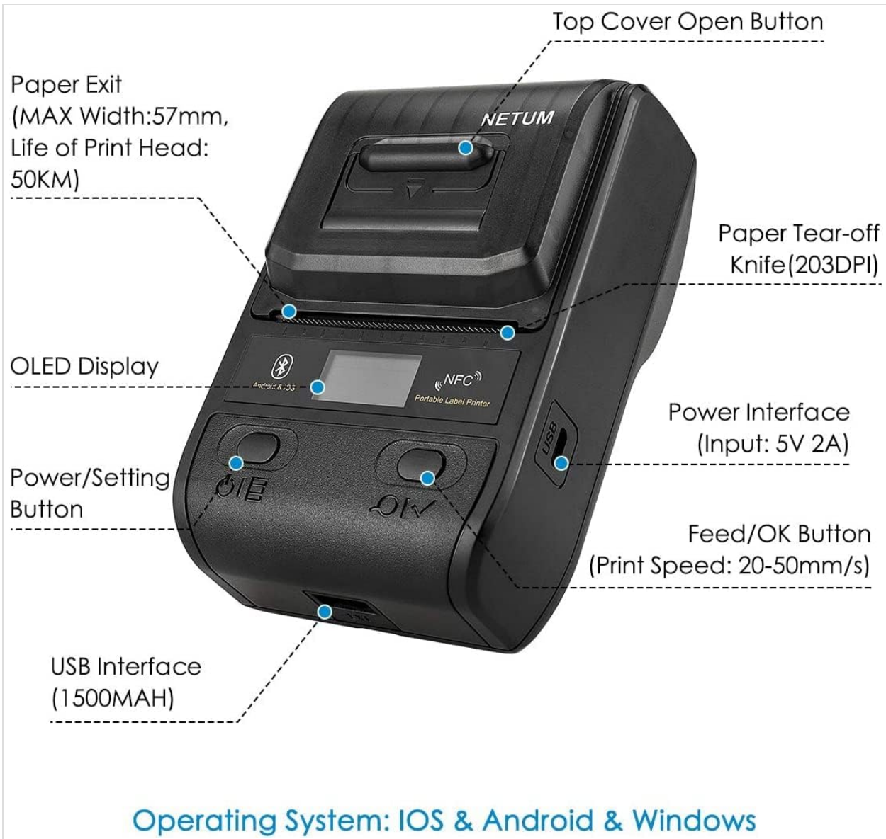
Image 2.2.1: Detailed view of the NETUM NT-G5 printer, highlighting key components such as the top cover open button, paper exit, OLED display, power/setting button, USB interface, power interface, and feed/OK button.
