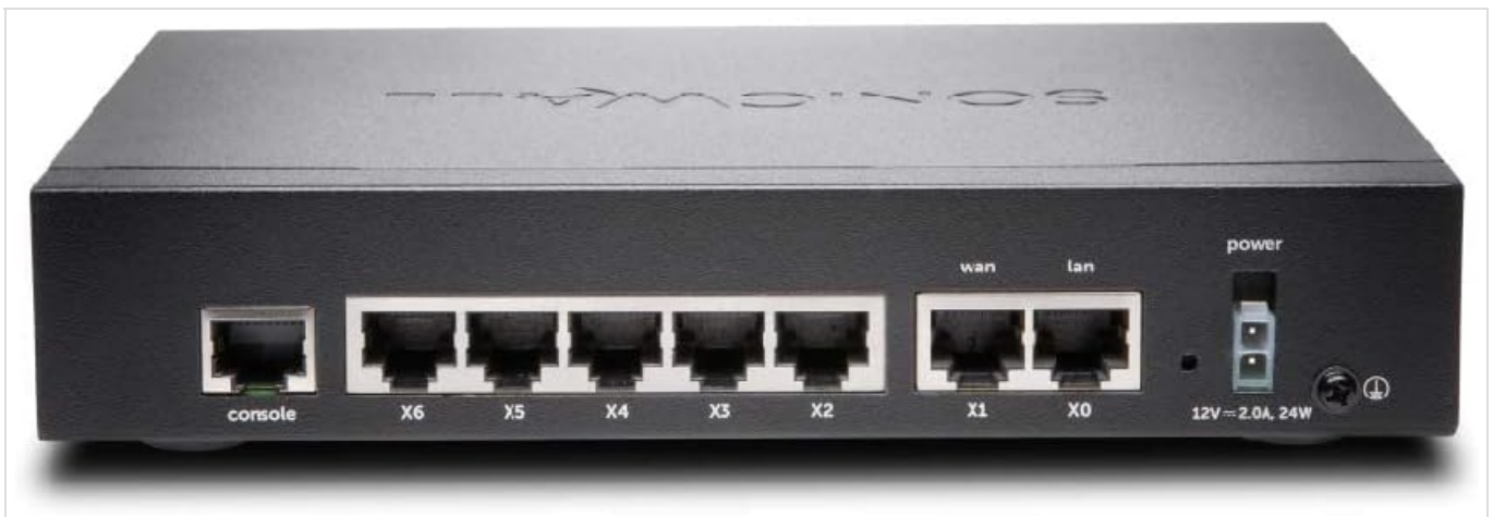
Image 1.2: Rear view of the SonicWall TZ400 appliance, displaying the console port, multiple LAN/WAN Ethernet ports (X0-X6), and the power input.
