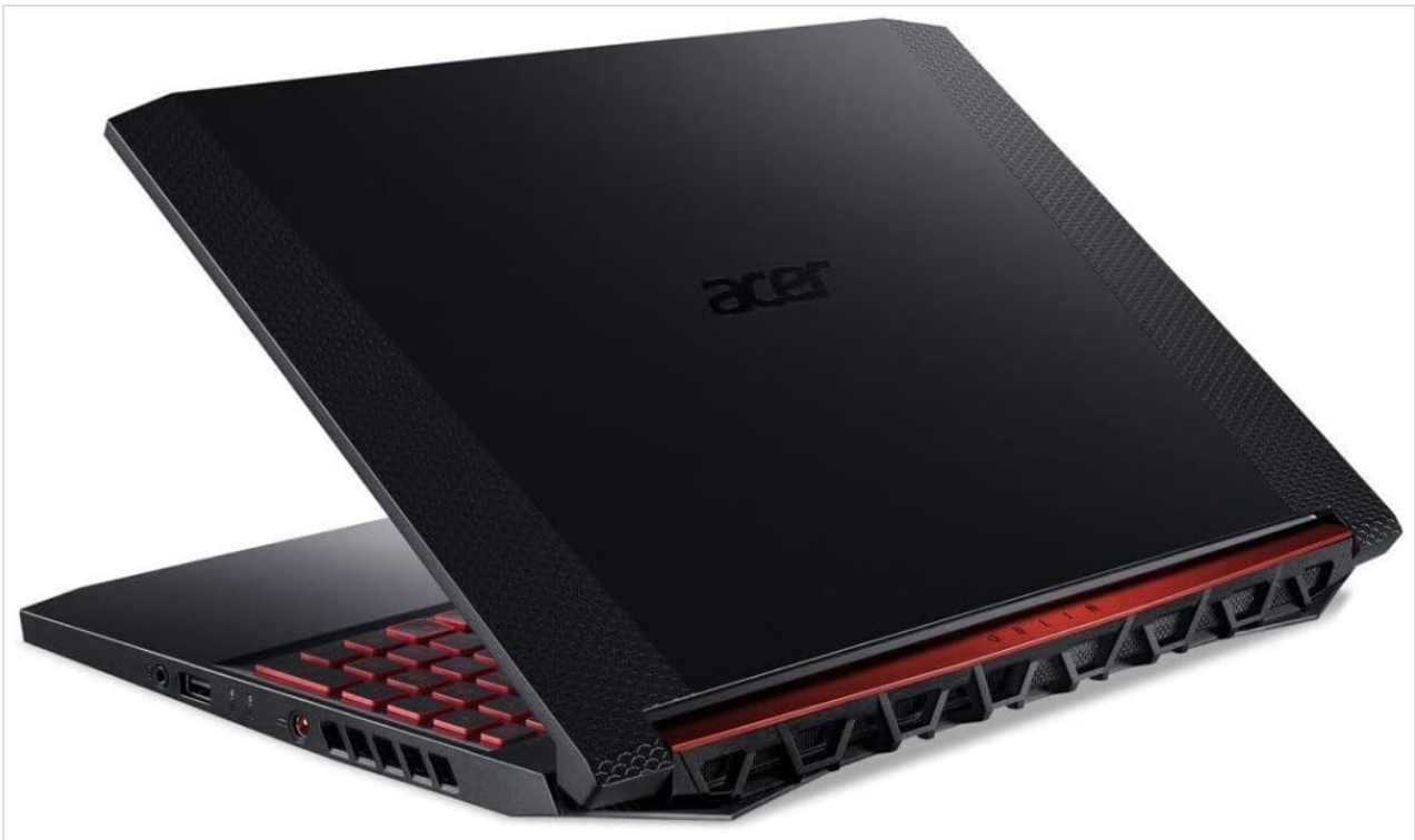
Rear view of the Acer Nitro 5 laptop, highlighting the prominent cooling vents designed to dissipate heat during operation.
