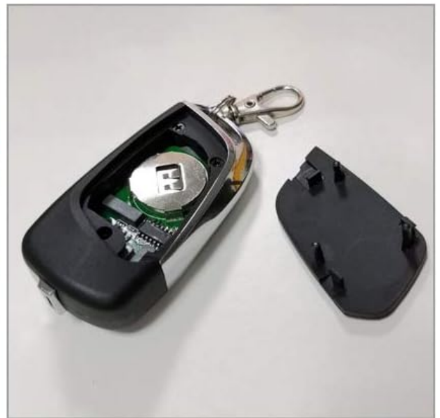
2. Take out the PCB (no need to un-screw) from the key fob shell & replace with new CR2032 battery.
