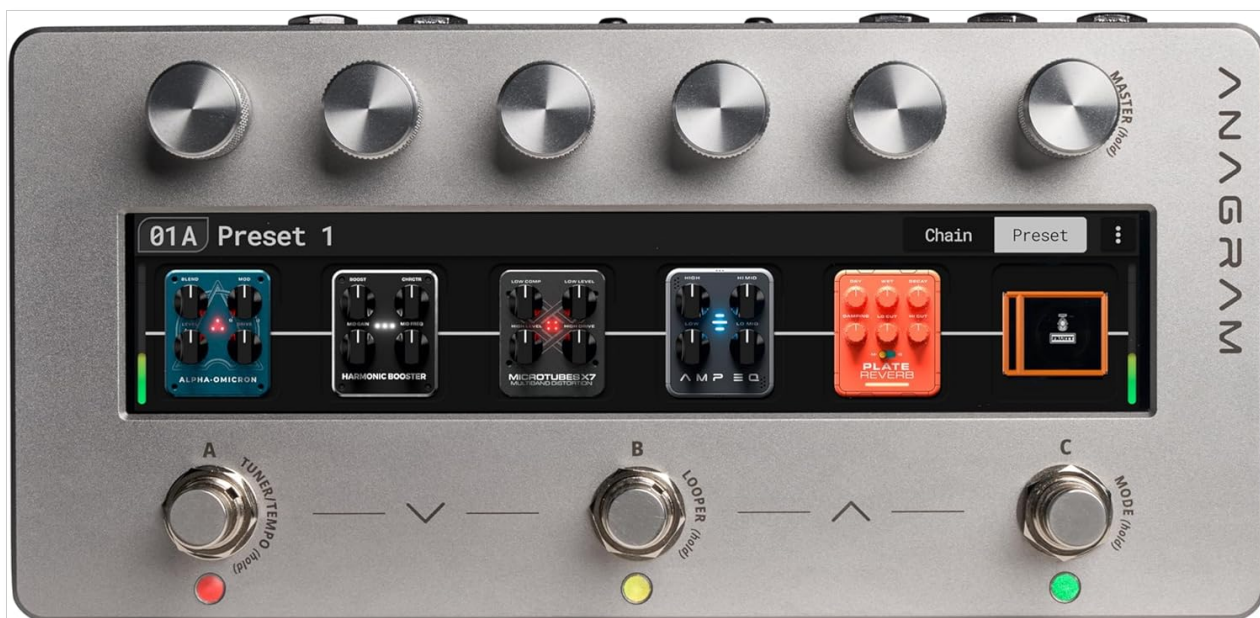
Figure 4.1.1: Front panel of the Anagram unit, displaying a preset chain with various effect blocks and the main control knobs and footswitches.
