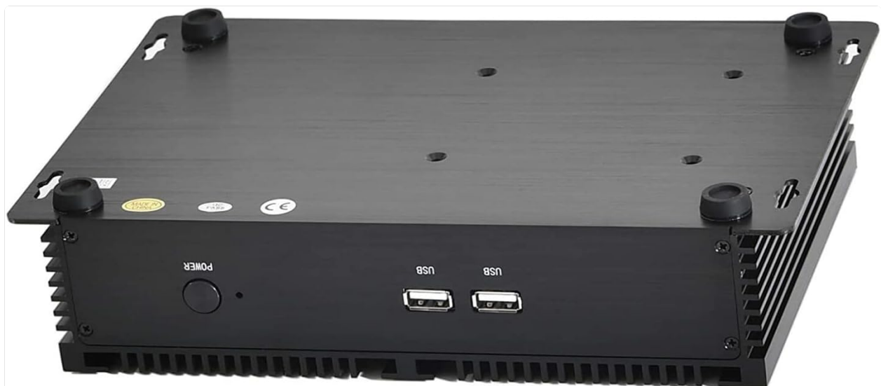
Image: Bottom view of the KINGDEL NC3000, showing the mounting points and rubber feet for stable placement.
