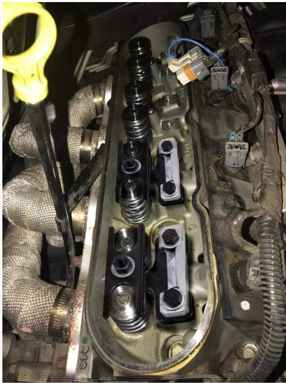
Figure 5: The tool installed on an LS engine cylinder head, compressing valve springs.
