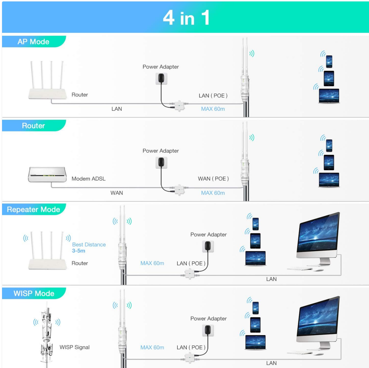
Figure 7.1: Diagram illustrating the four operating modes of the FLASHOWL AC600: AP Mode, Router Mode, Repeater Mode, and WISP Mode, showing typical network configurations for each.
