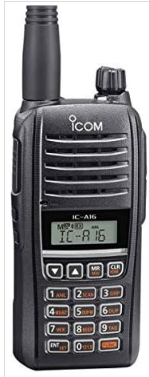
Figure 4.1: Front view of the Icom IC-A16B handheld transceiver, showing the display, keypad, speaker, and microphone.
