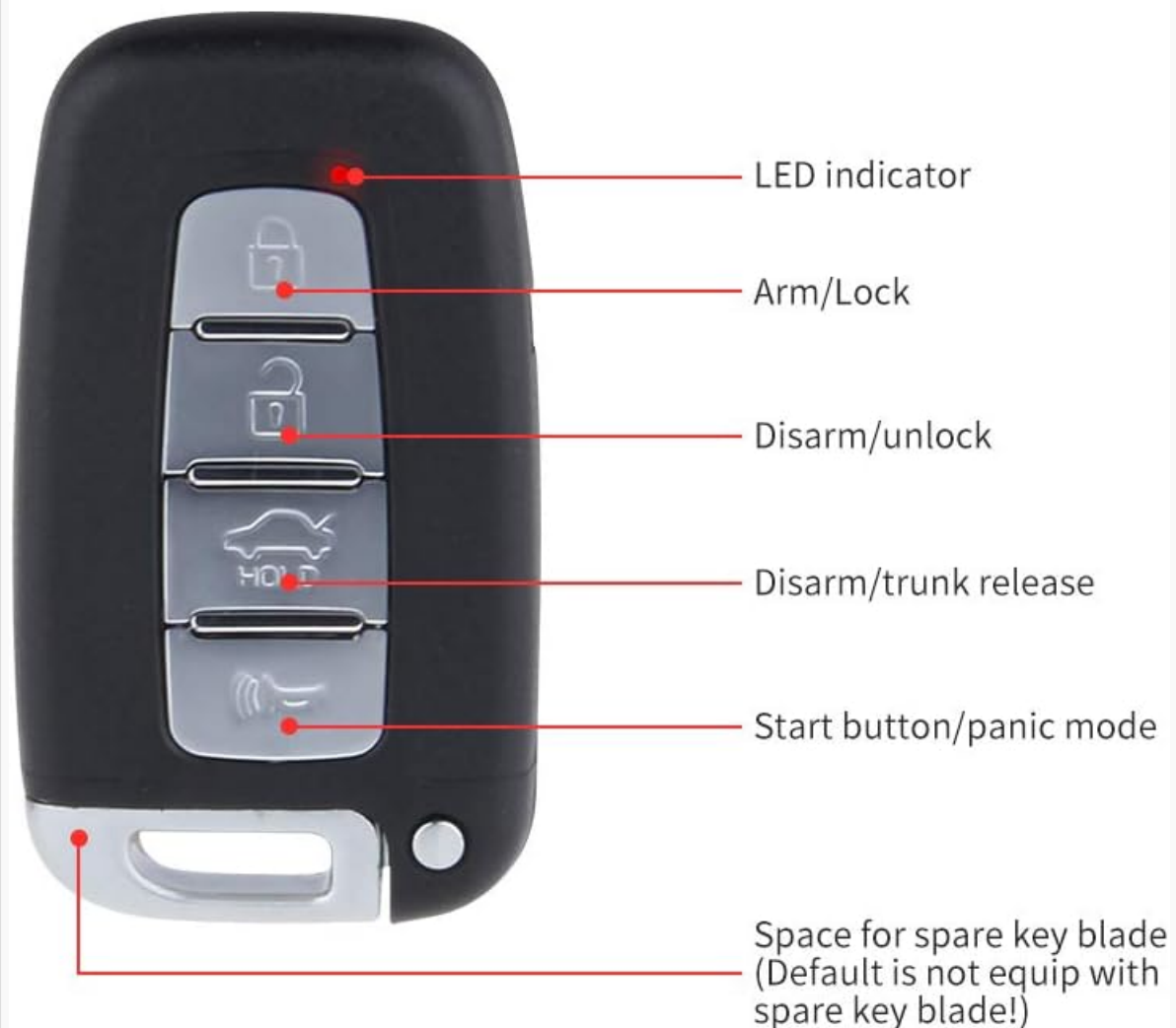
Figure 3: Key fob button functions.
