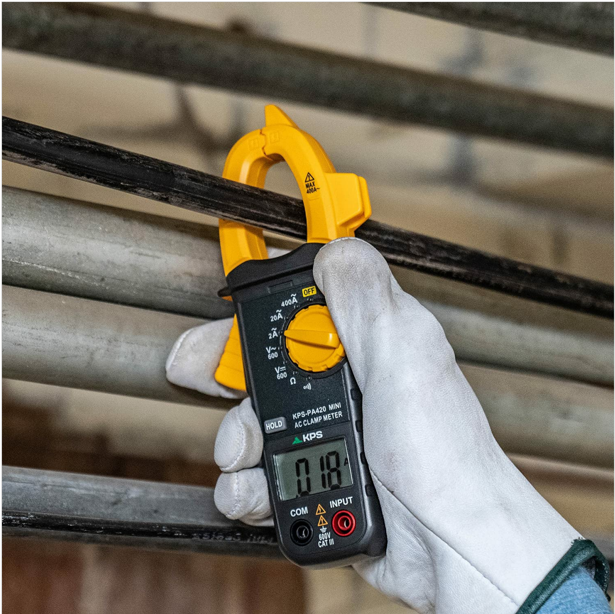
Image: A KPS-PA420 Mini Digital Clamp Meter being used to measure AC current by clamping its jaw around a single electrical cable.
