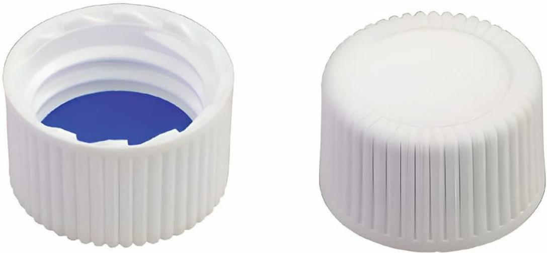
This image displays two views of the MACHEREY-NAGEL N13 Screw Cap. On the left, an open cap reveals the blue PTFE/Silicone septum lining the inside. On the right, the cap is shown in its closed, top-down view, highlighting its ribbed exterior for grip.
