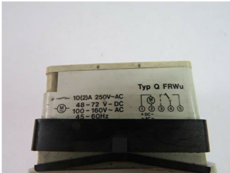
Figure 4: Detailed view of the product label, showing the model number (Typ Q FRWu), electrical ratings (10(2)A 250V~AC, 48-72V~DC, 100-160V~AC, 45-60Hz), and a simplified wiring diagram with numbered terminals (1-5).
