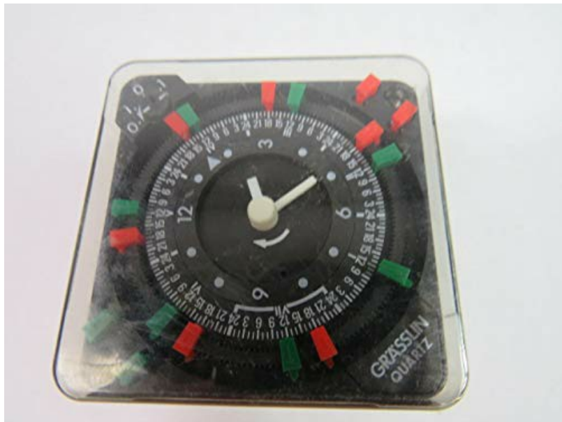
Figure 2: Close-up view of the timer dial. The dial displays 24-hour markings and features slots for inserting the red (ON) and green (OFF) programming pins, allowing for precise scheduling.
