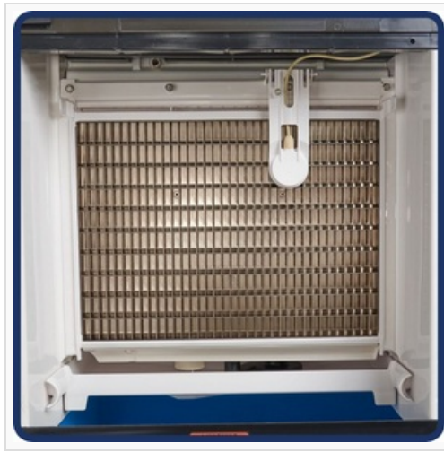
Figure 6.2: The evaporator plate is where ice forms and should be part of regular sanitation.
