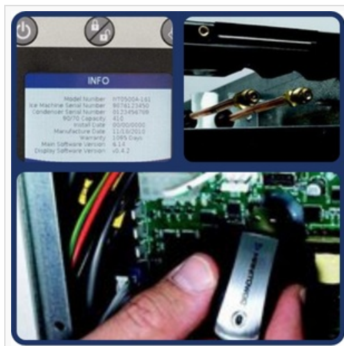
Figure 7.1: The machine's diagnostic capabilities allow for easy access to information and potential software updates via USB.
