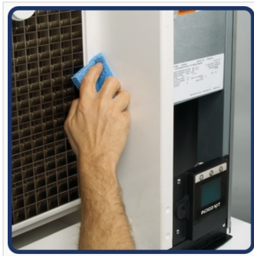
Figure 6.1: Regularly clean the exterior surfaces of the machine.
