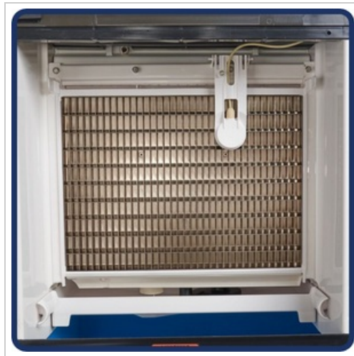
Figure 8: Internal view of the evaporator plate, which requires regular cleaning.
