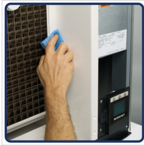
Figure 7: Cleaning the exterior of the ice machine.
