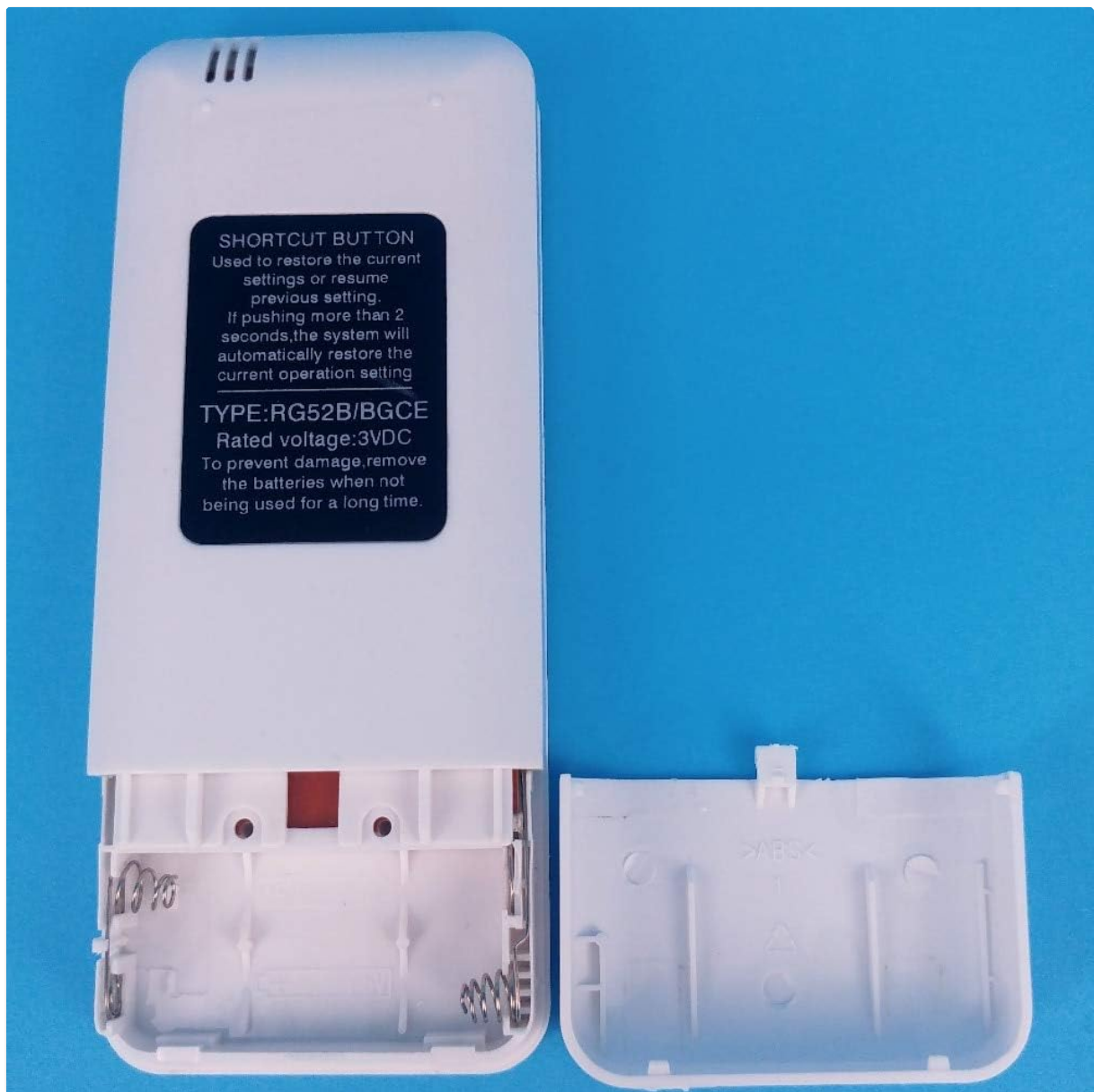
Figure 2.1: Battery compartment with cover removed, showing battery insertion.
