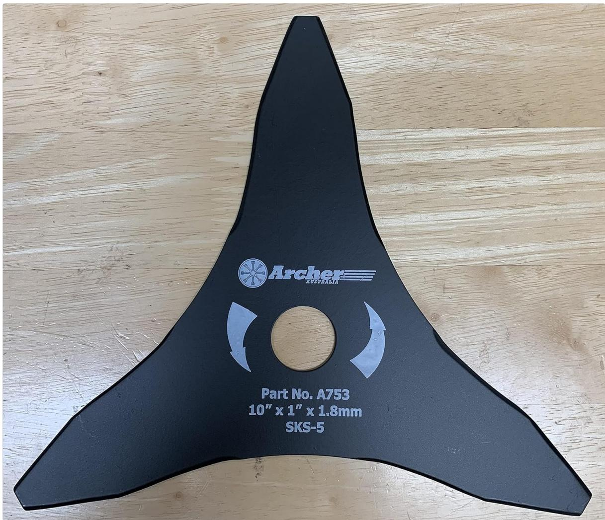
This image shows the Archer 10-inch, 3-tooth brush cutter blade. It features a central 1-inch arbor hole and is marked with 'Part No. A753', '10" x 1" x 1.8mm', and 'SKS-5', indicating its dimensions and material. Directional arrows for rotation are also visible around the arbor hole.
