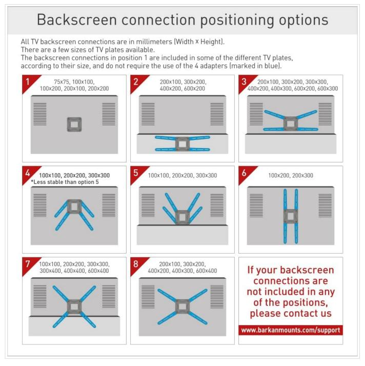
This diagram illustrates different ways the TV brackets can be attached to various TV backscreen connection patterns, including VESA 75x75 up to 400x400 mm.
