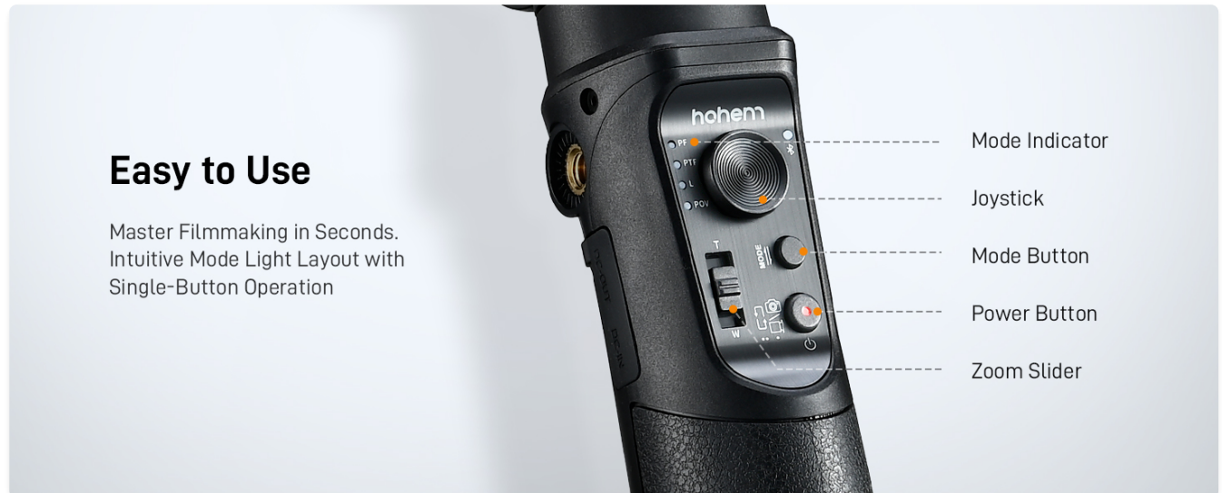
Figure 3: Gimbal controls including Mode Indicator, Joystick, Mode Button, Power Button, and Zoom Slider.
