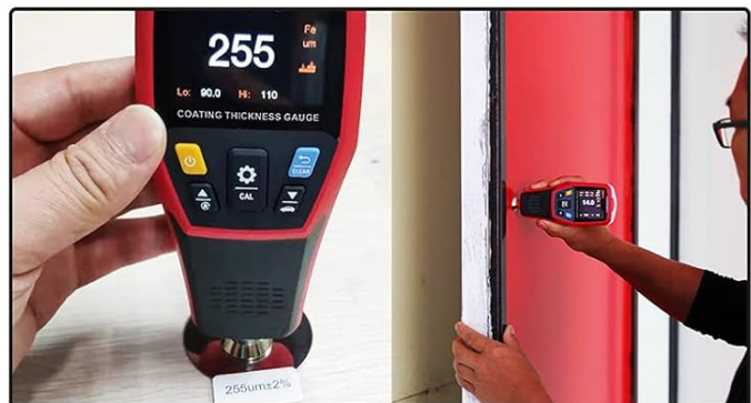
The probe automatically recognizes the substrate
