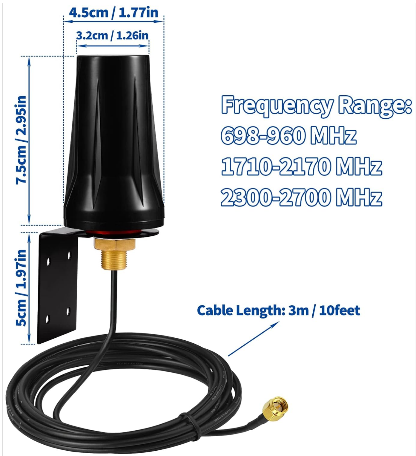
Figure 5.1: Detailed dimensions of the antenna and its supported frequency ranges.
