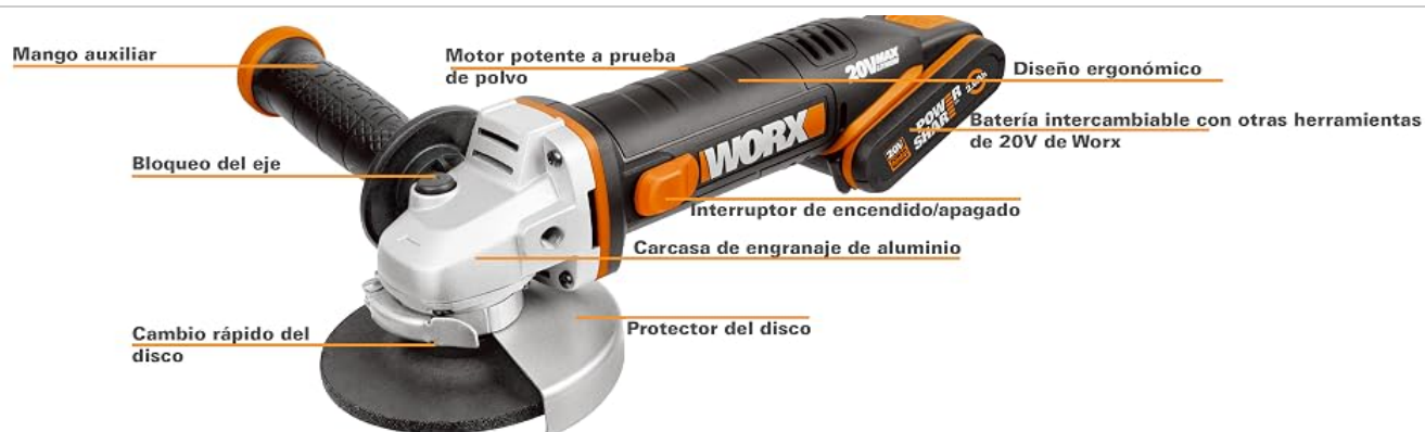
Image: Diagram illustrating the various parts of the WORX WX803.9 angle grinder.
