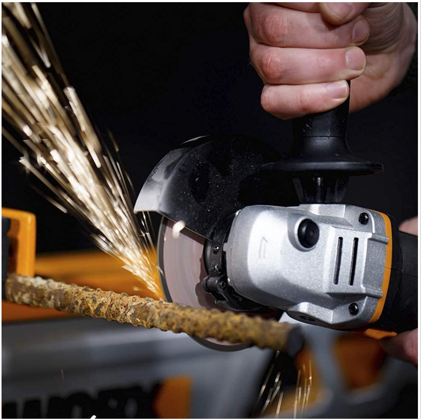
Image: An angle grinder grinding a rusty metal bar, creating sparks.
