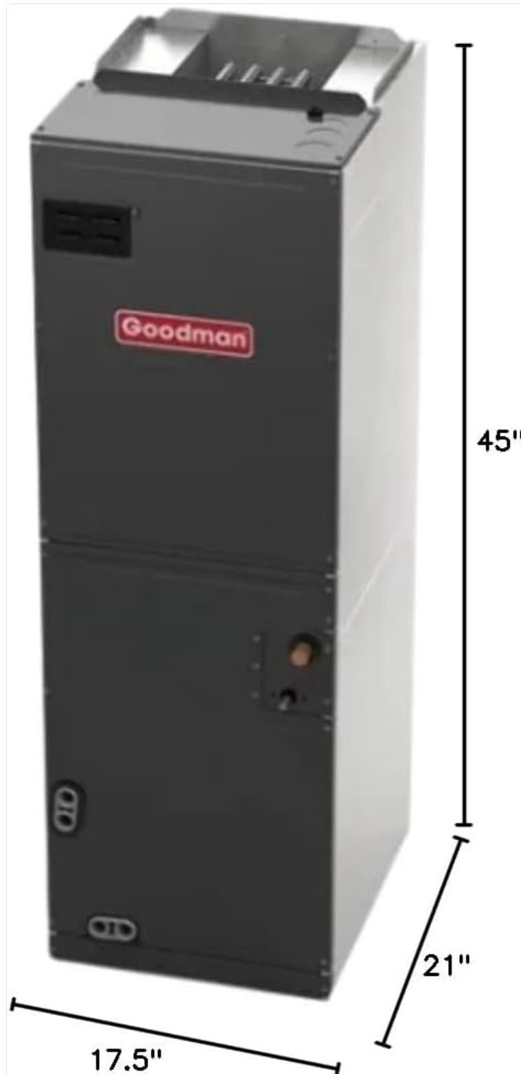
Image 4: Dimensions of the Goodman AMST24BU1300 air handler, indicating its height, width, and depth for proper installation planning.
