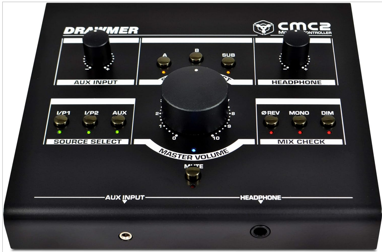
Figure 4.1: Front view of the Drawmer CMC2 Compact Monitor Controller, showing all knobs and buttons for input selection, speaker selection, master volume, headphone control, and mix check functions.
