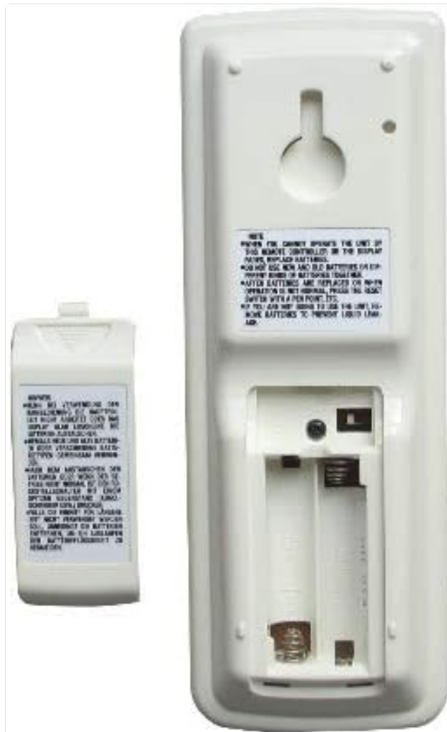
Figure 3.1: Rear view of the Fetcus remote control with the battery compartment open, revealing the two battery slots and a label with battery safety warnings. This image illustrates the correct orientation for battery insertion.
