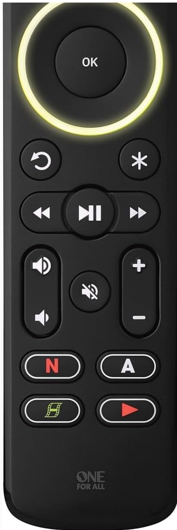
Figure 4.2: Remote with green light, indicating a different device is active.
