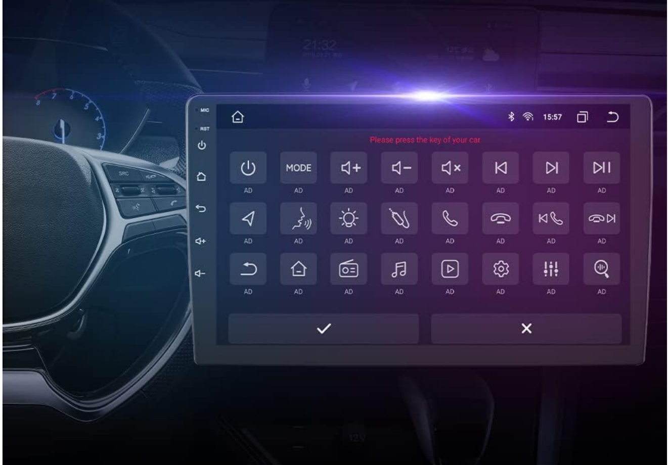
Image 5.2: Screen displaying the steering wheel control configuration menu, allowing users to assign functions to vehicle buttons.
